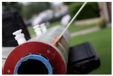
This looks like earlier pictures but here all the fitting and measuring is done and the fin pockets are epoxied in place. Internal fillets were added before final installation.
