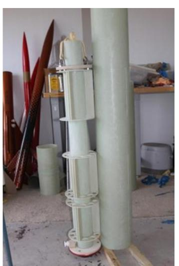
I started on a plywood fin alignment guide and then realized with the fin pockets inside the fins were self aliening. The front fins are less than 1/16" difference in tip to tip measurement. That is on a 24.5 inch fin span. The aft fins were also perfect when set in place but I still used square tube clamped to the front fins to make sure .
