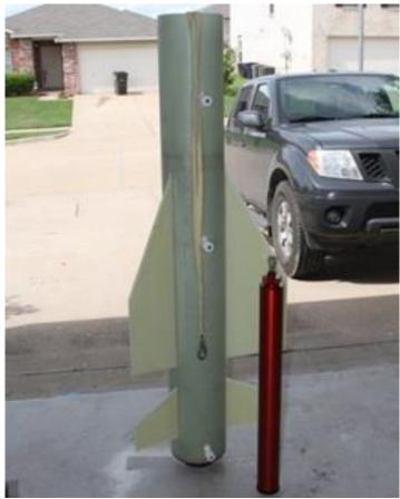
I added the aluminum ½" disc to keep the nose centered and a plywood bulkhead behind the washer. The machine screw was replaced with an eye-bolt a tether will connect here.
