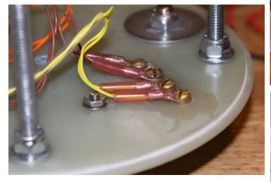
Below is top of nearly finished removable av-bay lid, the 5/16" rods are on 6.5 inch circles and the eye-bolts are only offset 30 degrees to keep the load on the rods and coupler. The fender washers on the rods reach to outside edge of the coupler.
